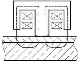
Figure1.1 Principle of magnetic induction method
