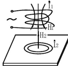
Figure1.2 Principle of eddy current method
